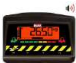
Overload situation: load too heavy
